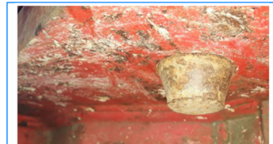
Photo of a retaining pin without a hole visible for the safety clip.
