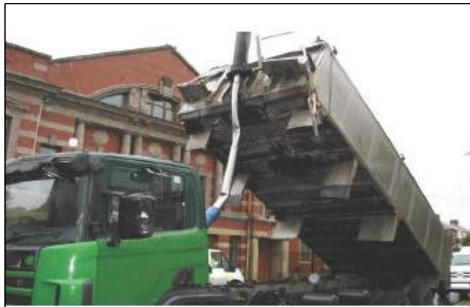
Photo (left): Result of Tipper equipment not correctly loaded after striking a bridge
