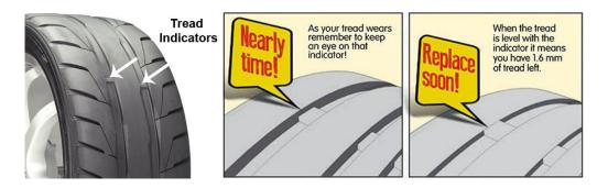
Premium tyre manufacturers mould TWI's into the design of the tyres' tread pattern. It's easily identifiable; it's made up of six or more small rubs across the bottom of the main tread grooves, which are usually 1.6mm to 2mm above the base of the groove. The legal limit of 1.6mm is reached when the tyre is worn to the level of the tread wear indicators in the main groove — as soon as this happens, the tyre should be replaced.
