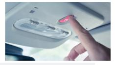
There is no need to check if your eCall is working, as the system will carry out a self-test each time the vehicle is started.
