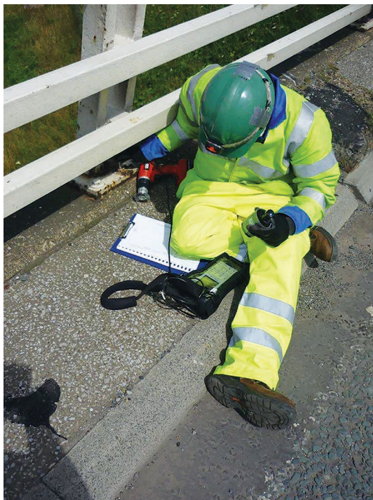
Figure 7.8 Ultrasound testing of bolt length and condition (courtesy Mistras Group Ltd)
