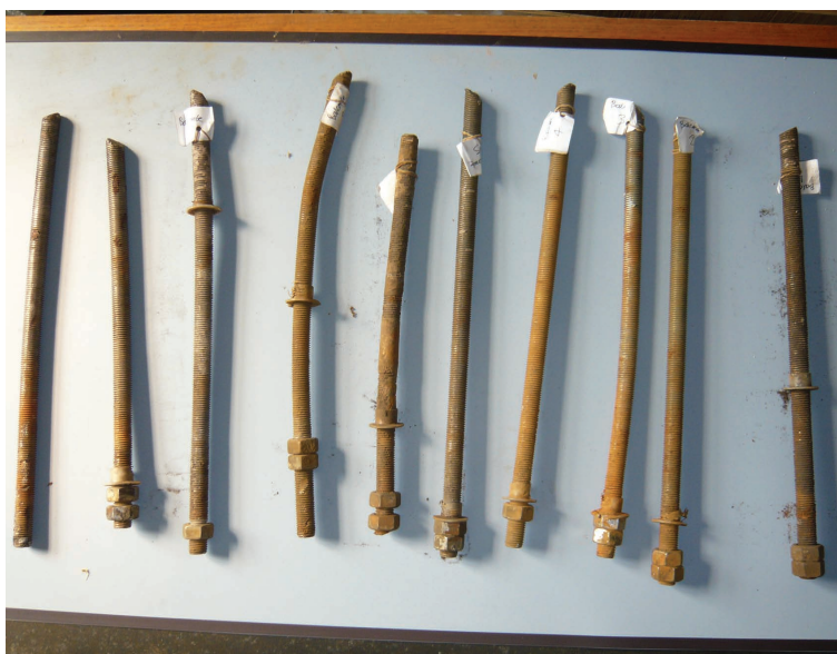
Figure 7.1 Missing studs that had fallen to the ground and were found by track patrollers over a seven-month period before the failure (courtesy RAIB)
