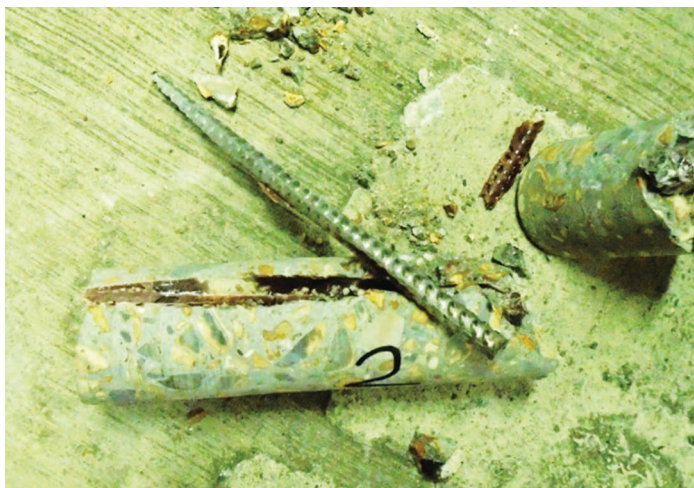
Figure 7.7 A section of dowel that came out clean upon breaking the core open, indicating that the bond between dowel and concrete was ineffective (courtesy Southampton City Council)
