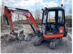
At this point his injuries were not too severe because he was wearing the correct safety boots. He then tried to track the machine back off his foot by reaching into the cab and pulling the tracking control lever. Unfortunately, he moved the lever in the wrong direction causing the machine to track further forward onto his leg. He managed to attract the attention of a General Foreman nearby who raised the alarm and called for an ambulance.
