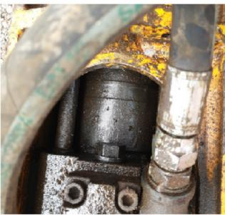
The employee sustained the injuries as he attempted to relieve excess hydraulic pressure known as 'Hydraulic Lock' which prevents the hydraulic hoses being attached to the excavator couplings. This can occur when any hydraulic attachment is:
