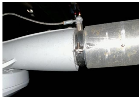
Photograph 1. Lanyard incorrectly fitted
