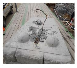
Whilst unloading a batch of blocks from a flatbed, the lifting point came away from the concrete as the block went under tension ready to lift. (See photos below)
