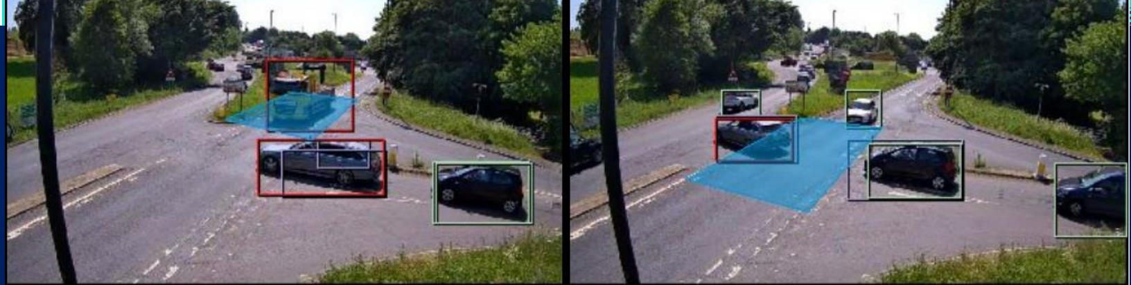
Above: Dangerous Driving (Near Miss) caught by AI, the system detects a vehicle pulling out in front of an HGV, and then stopping in the live lane, forcing another vehicle to stop.
