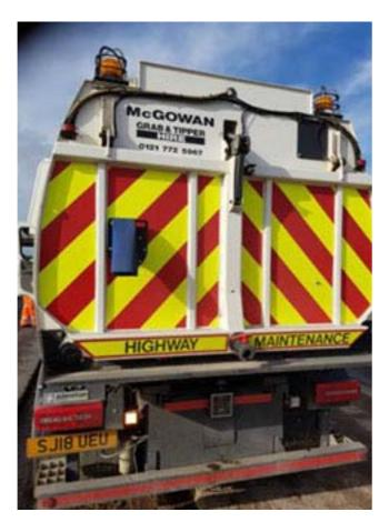
If the vehicle needs to get closer to an obstruction the driver can turn a key to briefly override the system but it will immediately default to "on" so can't be permanently deactivated.
