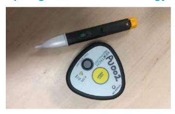
All engineering staff on the BMJV project have been trained and issued with Voltage Detector sticks and proving units. Before any Cat and Genny survey work is carried out, Proving of electrical safety is carried out.
