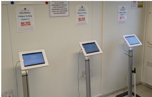
Touch screen kiosks used to measure impairment due to fatigue on site.
