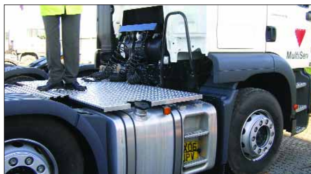
Figure 2 A single level platform forms the catwalk and also covers the top of the fuel tank. There is a good handhold and access steps are set in the fuel tank. These will need to be kept clean from any diesel contamination.
