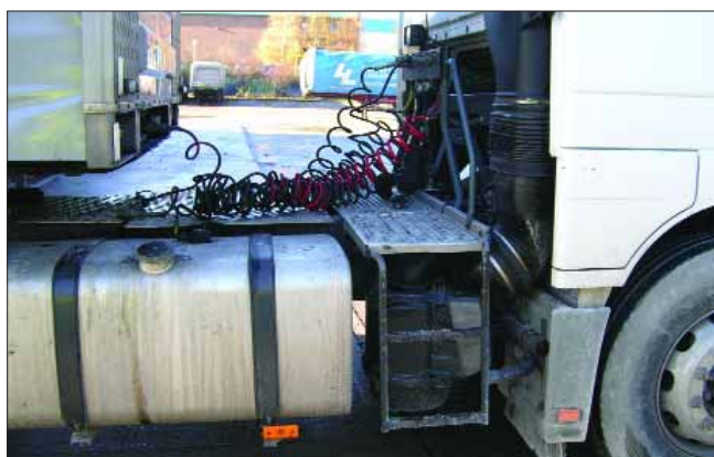
Figure 1 Earlier version of the catwalk with smaller area for the feet and changes of level that are more likely to cause operators to trip and fall.
