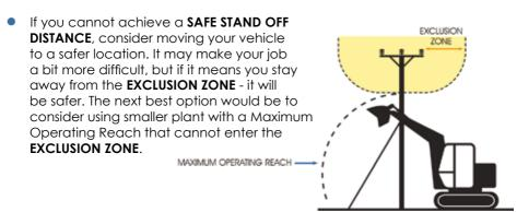
You may not be able to achieve either of these options, so, as a last resort, if you cannot avoid operating large items of plant in the vicinity of lines, you MUST make sure that the plant is fitted with restraints to ensure that the EXCLUSION ZONE cannot be entered. These restraints may be electrical or hydraulic systems fitted to the plant, or mechanical devices such as chains.
