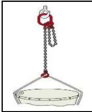
Two Leg Sling, One Leg Used (De-rate as applicable)
