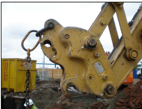
Figure 3 – Hitch tilted backwards with master link subject to bending
