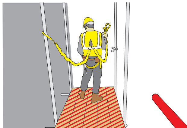
Figure 68: Double lanyard system using two separate fall arrest lanyards.
