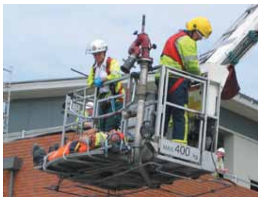
Figure 81: Recovery from height by emergency services. Shows the emergency services using a MEWP to recover an accident casualty from height. However rescue plans must not rely upon the emergency services to recover a person suspended by personal fall protection equipment.
