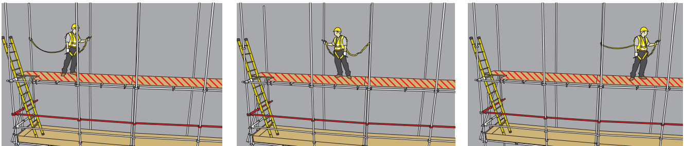
(ii) To traverse, double lanyards are used to remain continually attached, ideally to the inner standards or ledgers.
