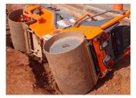
In April 2019, on schemes across the Smart Motorway Programme, there were three incidents involving narrow (800mm) ride-on twin drum rollers overturning.
