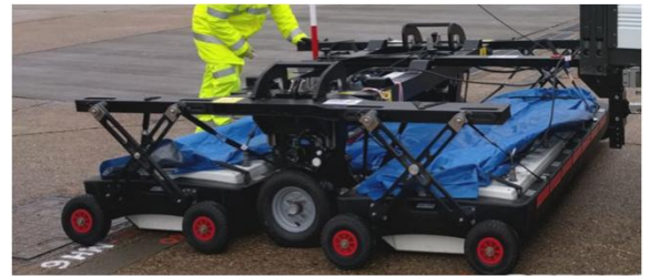
Radar survey equipment to locate services
