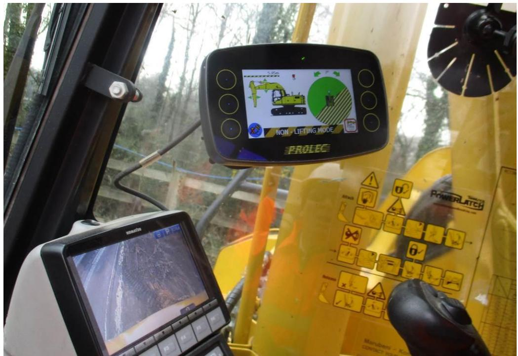
Prolec height and slew restrictor system fitted to plant
