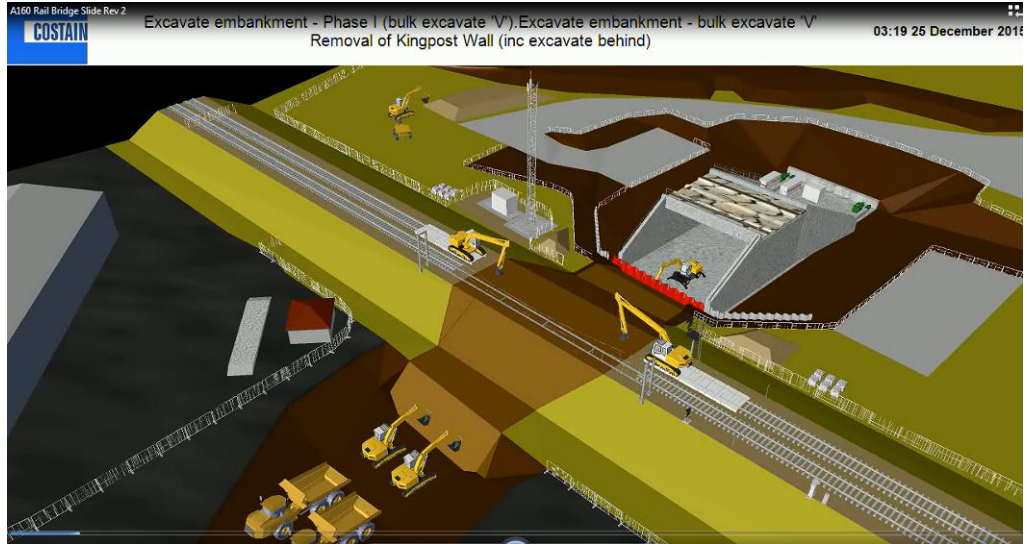
Still from DVD model of bridge slide used in bridge push induction
