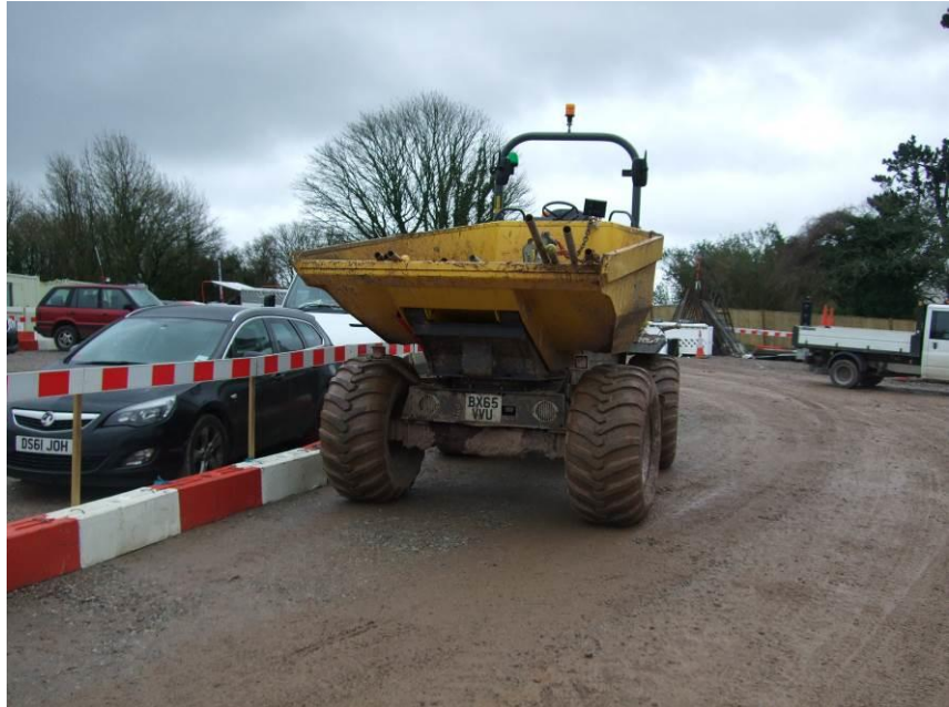
9t swivel dumper with forward view camera
