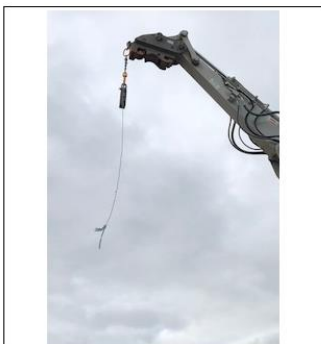
Correct Position – accessories hanging freely from quick hitch
