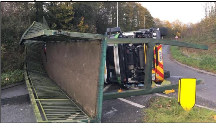
On the 8<sup>th</sup> November 2017 at J13-14 of the M60, a lorry loader was moving forward with the boom extended. The crane impacted an unidentified gantry which received superficial damage and causing significant damage to the loader.
