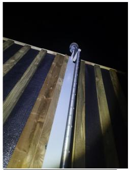
3m High surveying Environmental Barrier with GPS Head Unit Attached
