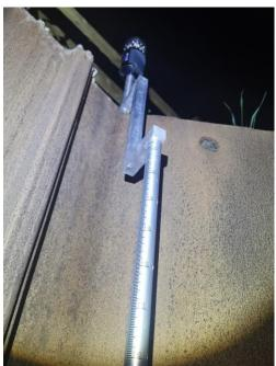
3.2m High Surveying Sheetpiles using standard Prism
