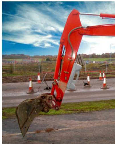
EZiDIG magnetically mounted on to the excavator boom.
