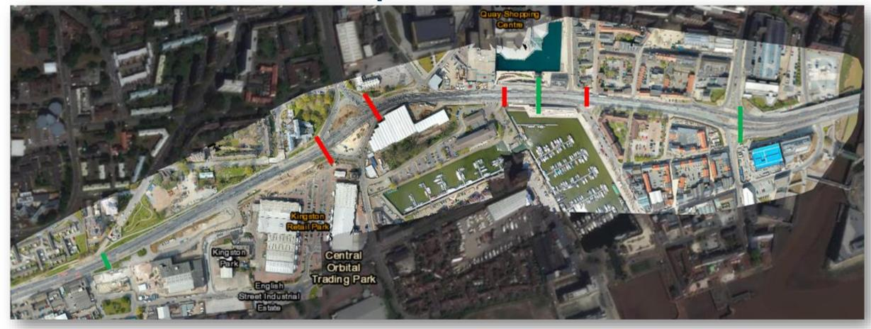
To allow works to progress of the construction of a city centre underpass we were required to permanently close a number of existing pedestrian crossing points (marked in red) and establish pedestrian diversion routes. This approach was extensively consulted & agreed on during the ECI phase
