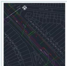
Photo of Plans for the Cores with Nation Grid cables (Purple) added.
